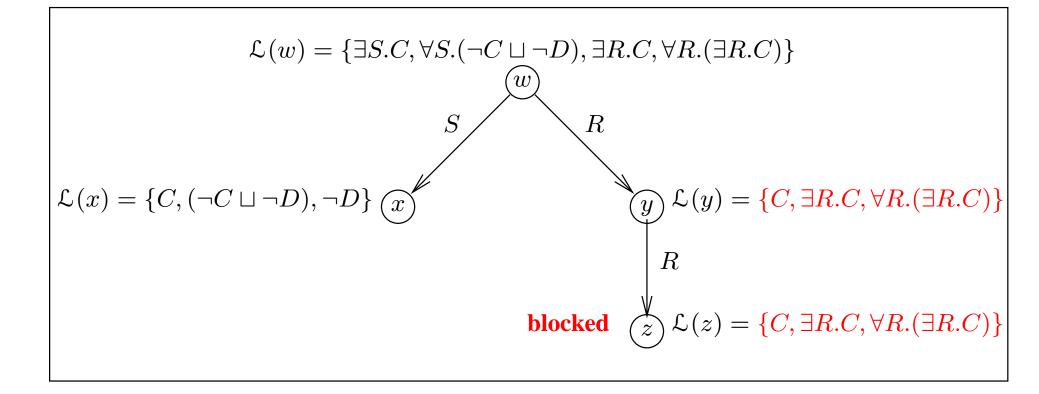
Test satisfiability of  $\exists S.C \sqcap \forall S.(\neg C \sqcup \neg D) \sqcap \exists R.C \sqcap \forall R.(\exists R.C)\}$  where *R* is a **transitive** role
