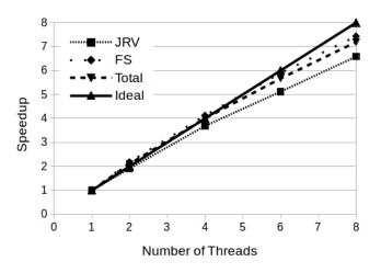
Fig. 6. MAST scales very well on a single socket using the optimisations. Here the results are for selecting 100 features from a datset of 1,000 examples and 1,000 features.
