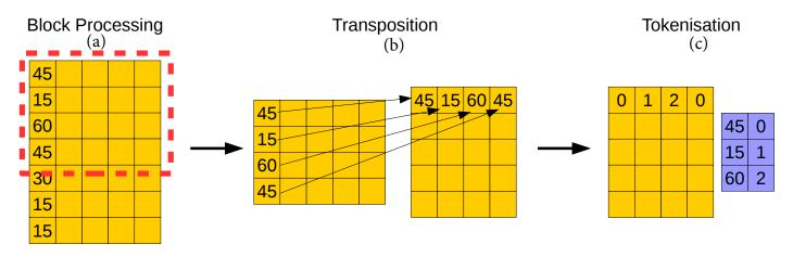
Fig. 1. Data is preprocessed for tokenised arrays in three steps. First the data is read in blocks. Those blocks are then transposed so that the consecutive values of the same feature are in contiguous blocks of memory. Finally the feature values are converted into "tokens" which are consecutive integers.
