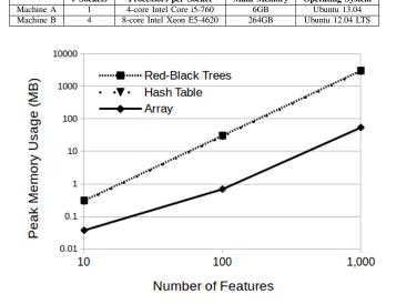
Fig. 2. The peak memory usage with arrays was consistently an order of magnitude lower than with either of the alternative storage methods.
