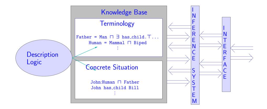
A Description Logic - mainly characterised by a set of constructors that allow to build complex concepts and roles from atomic ones,
