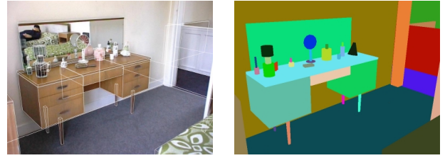
Figure 8: An off-screen frame-buffer (right) is used to store the identification number for each primitive in the model (left).
