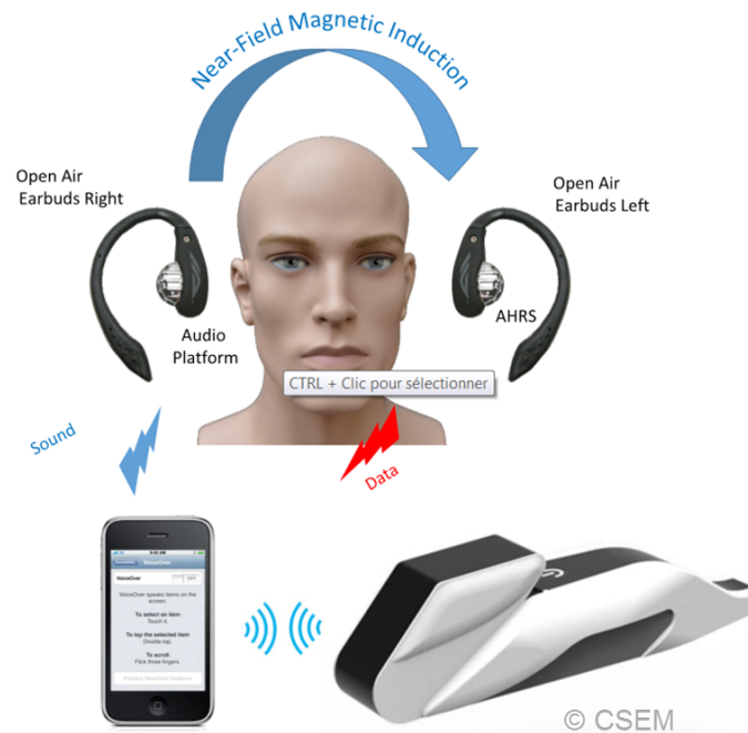
FIGURE 3 The complete INSPEX system for the VIB use case.
