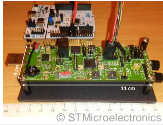
Fig. 8. The MEMS ultrasound sensor (ST Microelectronics).
