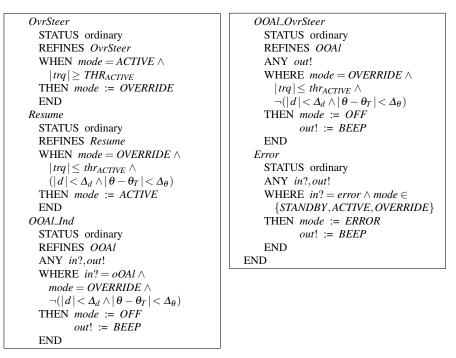
Fig. 5 Enhancing the mode level lane centering control to fully continuous control. Second part.
