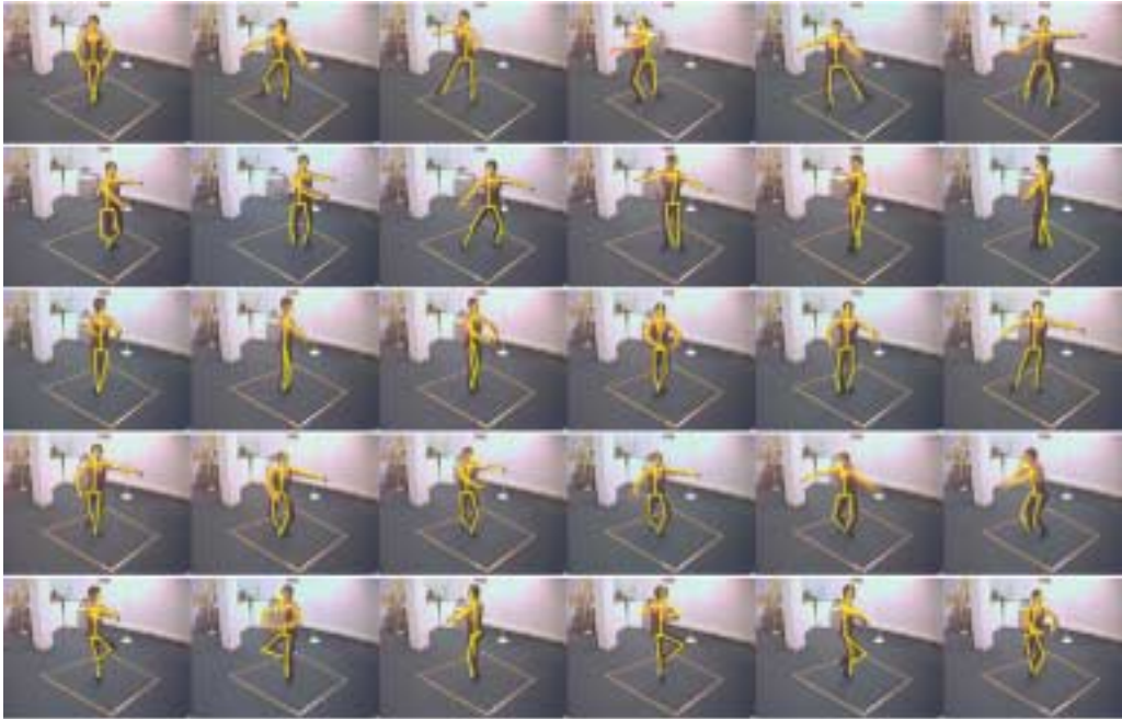
Fig. 10. Tracking the second dance exercise using a VLMM with a maximal history of 20 frames and 1000 particles.
