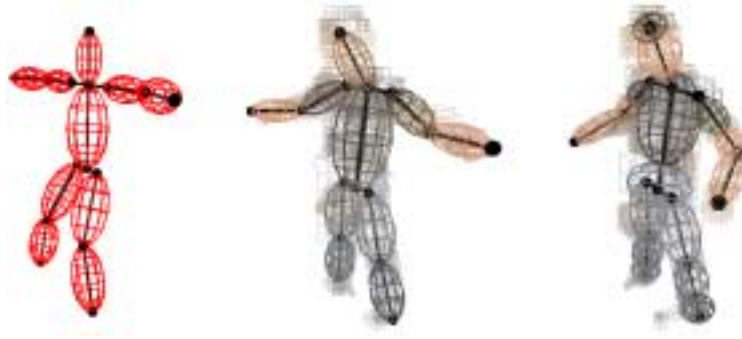
Fig. 7. Automatic acquisition of the blobs models over 20 frames. Note that the initial global position and orientation of the model are computed from the mean and the principal axes of the voxels distribution.
