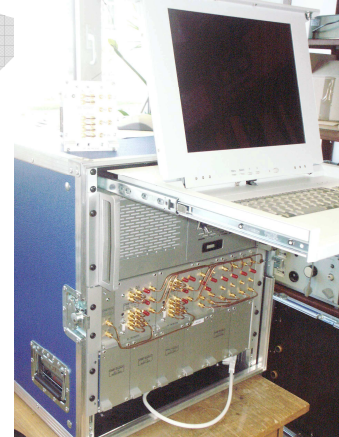
Fig. 2. Real-time UWB MIMO channel sounder
