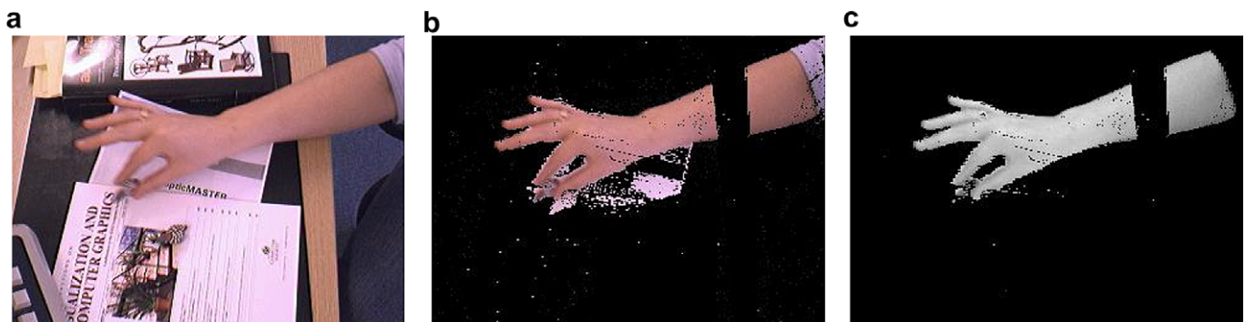
Fig. 3. Image processing: (a) Original image, (b) background subtraction and (c) skin detection.
